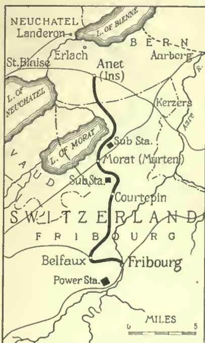
FIG. 475 ELECTRIFIED LINES OF THE FRIBOURG-MORAT-ANET RAILWAY
